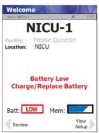
Battery Low. Place meter into charging/docking station.
