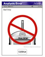
Occurs after test strip insertion or during analysis. Insert another strip and repeat the test.
