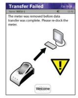
Meter was removed before data transfer was complete. Re-dock the meter.
