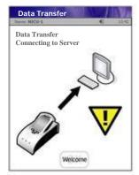
Meter is unable to connect to the transfer computer. Contact your Point of Care Coordinator for assistance.
